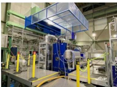
Single-cylinder test engine
